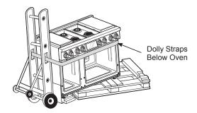
4 Transport the range on the furniture dolly close to its final location, tip the range back to level, and carefully remove the dolly.
