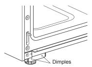
Insert the provided screws through the holes in the leg cover assemblies to secure them in place.
