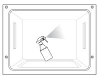
5 Fill and spray or pour the remaining 10 oz or 300 ml of water onto the bottom center of the oven cavity. The indentation on the oven bottom should be fully covered to submerge all soils. Add water if necessary.
