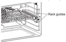
3 Once the rack is secured in the back, pull the entire rack forward until the rack locks into place.
