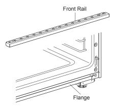
3 Use the 3 screws provided to secure the front rail to the flange.
