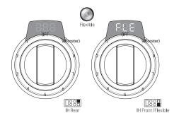
In Flexible mode, both cooking-element sensors are turned on. When larger cookware is placed on the cooktop, both elements operate simultaneously.
