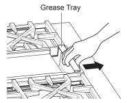
Carefully lift the grease tray up to remove it.
