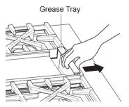
2 Carefully lift the grease tray up to remove it.
