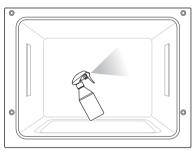
5 Fill and spray or pour the remaining 10 oz or 300 ml of water (for right oven) and 8 oz or 240 ml of water (for left oven) onto the bottom center of the each oven cavity. The indentation on the oven bottom should be fully covered to submerge all soils. Add water if necessary.
