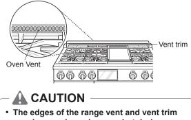
The edges of the range vent and vent trim are sharp and may become hot during operation. Wear gloves when cleaning the range to avoid burns or other injury.
