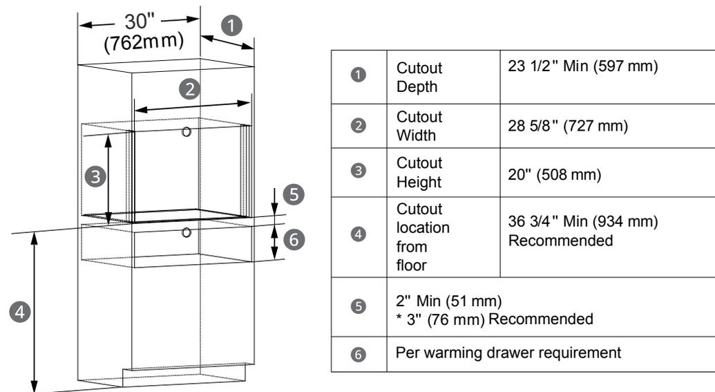
**NOTE:** Additional clearances between the cutouts may be required. Check to be sure the oven supports above the warming drawer location do not obstruct the required interior depth and height. See warming drawer's installation instructions for details.
