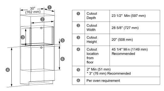
NOTE: If you are replacing an electric double oven with the combined installation of a wall oven and a speed microwave oven, use the dimensions shown. The middle rail separating the two openings may need to be larger than the 2" minimum shown.
