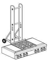
Transport the rangetop on the furniture dolly close to its final location, tip the rangetop back to level, and carefully remove the dolly.
