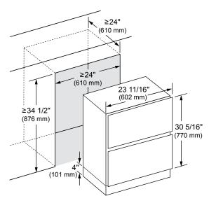
\*A minimum 4" (101 mm) finished return that matches the cabinet exterior is recommended on all sides and at the top of the cutout opening. The shaded area will be visible after installation.
